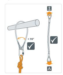
Performance and ultimate strength will be reduced by larks footing / choking around anchor points, storage and ageing due to use, etc. (list not exhaustive).
